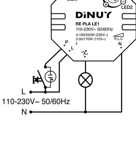
Example: replacement of a two way switches installation by a dimmer and pushbuttons
